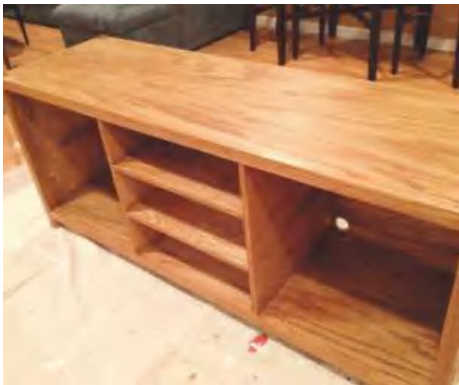
STEP 22. Cut holes in the back for wire access. Apply two coats of light honey stain followed by three coats of matte polyurethane
